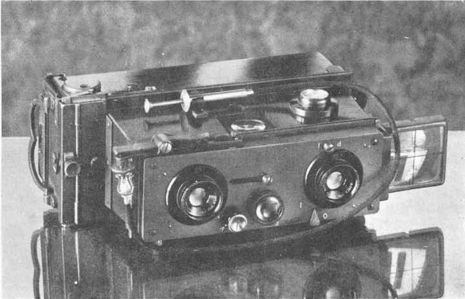
Model 4 Verascope showing Saphir f.8 lenses
