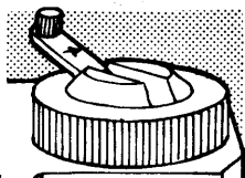
The rewind crank of the Zenith TTL.
