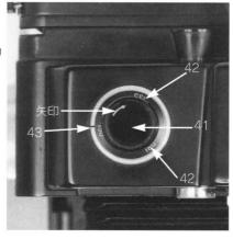
till it completely stops at the back by rotating the focusing knob (30). Then rotate the cam change dial (41) towards the arrow mark on the dial and match the focal length of the lens (42) to the index (43). At this time, the overlapped images in the rangefinder must coincide at infinity.
