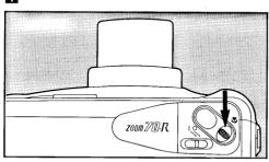
Press the macro button (♠) to engage the Macro mode, and the lens moves forward. To cancel the Macro mode, just move the zooming lever to the left (♠♠♠) or right (♠). The ordinary shooting mode is then restored.
