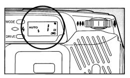
When the LCD panel is as shown above, the camera is in the Auto and Single-Flame Shooting modes. These modes are used for ordinary picture-taking situations. The flash fires automatically in dimly lit places.
