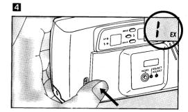
Close the back cover. The film automatically advances to the first frame.
