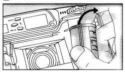
Open the back cover, and remove the cartridge from the chamber by pulling on its top with your fingertip as shown.
