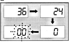
■ After you have exposed the last frame of the roll, film rewinds automatically. Then, the motor stops, and (OD) flickers as shown to indicate end of rewind
