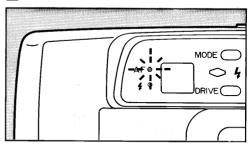
$\blacksquare$  The macro shooting range is 0.6  $\sim$  1 meter (2  $\sim$  3.3 ft). Press the shutter release button halfway, make sure the green lamp ( AF ) glows, then release the shutter.
