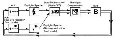
• Pressing the red-eye reduction flash button ( \$ ) @ in the Auto or Daylight-Sync mode alternates the normal mode (indicated by black line) with the red-eye reduction flash mode (indicated by red line).
