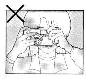
When shooting, hold the camera securely with both hands. Keep the camera as still as possible, and gently press the shutter release button. (If pressed forcefully, the camera is likely to shake, and the picture will be blurred.) Try to brace your elbows against your body, or support yourself and the camera against a stable, stationary object, such as a wall.
