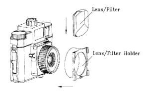
There is a Lens/Filter Holder available as an optional accessory. Lenses/filters for different effects, also available as optional accessories, can be inserted into the Lens/Filter Holder. The Lens/Filter Holder is then installed by being slid over the bezel of the lens of the camera.
