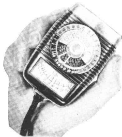
With baffle up, meter reads reflected light directly.
