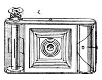
Take off the back by sliding the lock D. Raise up the spool key E which is hinged, and insert an empty spool in the receiving chamber, then close down the key, seeing that it engages in the
