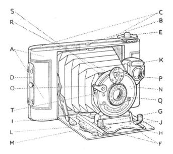
On receiving the WATCH POCKET CARBINE it should be opened by pressing the catch B, and then carefully compared with the illustration, so that by means of the letters the names of the various parts may be identified to assist in understanding the directions for working.
