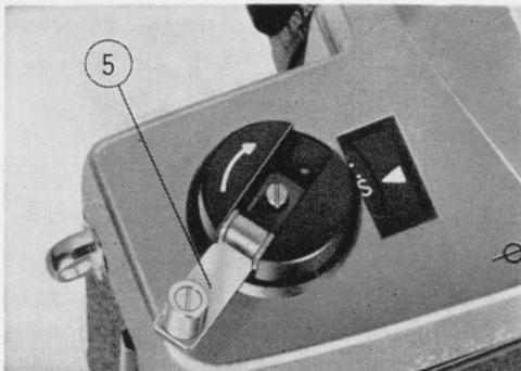
in the direction of the arrow. Rewind smoothly and at an even speed **BECAUSE** erratic or too rapid rewinding may cause static electricity marks on the film.
