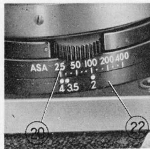
There are 13 click-stopping ASA film speeds from 25 to 400, with the dots between numerals indicating intermediate film speeds.
