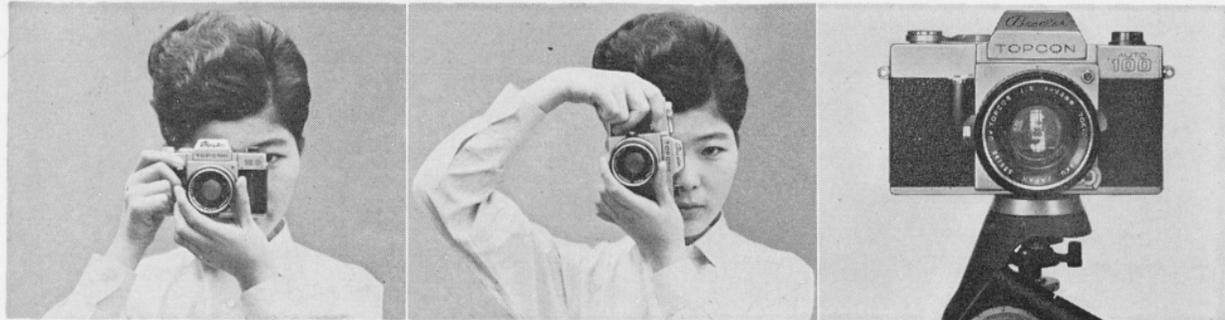
against the body for support and the camera should also be pressed against the forehead to minimize camera movement.
