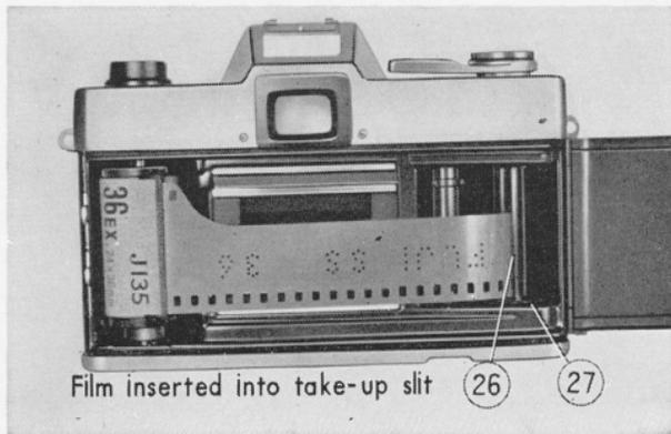
will go, and insert a fresh film cartridge into the empty film chamber. The leading end of the film should be pointed in the direction of the take-up spool slit (26).
