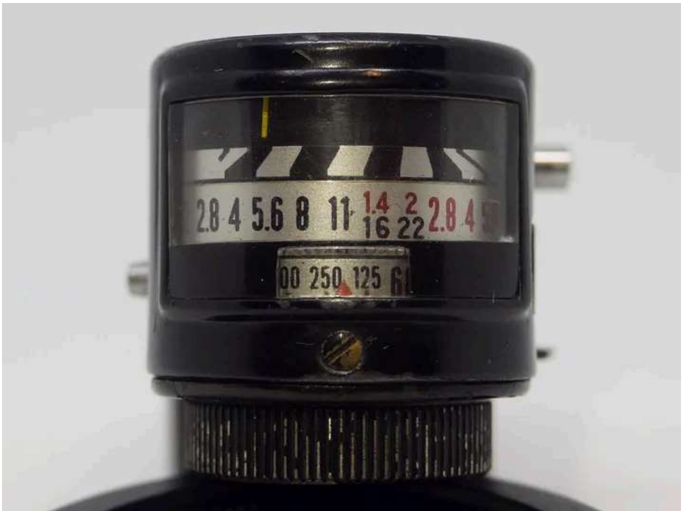
The Exposure Window is located at the top of the Olympus Pen F Exposure Meter.
