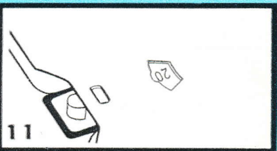
11. Move camera out and in twice. Number 20 will now appear in Counter Dial Window, showing you have 20 pictures to take. Pull camera out a third time and take your first picture.
