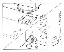
The Mamiya 7 II features an X synchro flash terminal and its lens shutter system permits flash synchronization at all shutter speeds.
