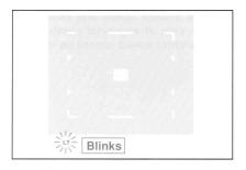
★ Blinking "LT" indicates under-exposure: rotate the aperture ring until the LED stops blinking to increase exposure.
