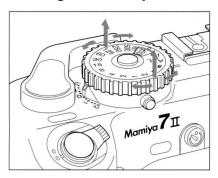
Set the film speed of the film being used by lifting up the outer rim of the shutter speed dial and rotate it until the correct ISO value appears in the window.
