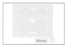
★ When "▶" LED blinks, it indicates overexposure. Rotate the aperture ring to stop down to a smaller f/stop until an LED indicates proper exposure.
