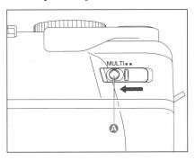
While pressing the lock release button (A), move the lever in the arrow direction to the multiple exposure position.
