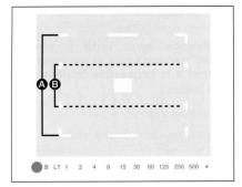
Within the viewfinder the subject area covered is indicated by the visible bright frame. Parallax is automatically compensated for according to the subject-to-lens distance.
