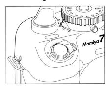
Press the shutter release button when you have focused and determined composition.
