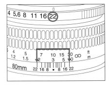
The depth-of-field varies according to the aperture. The smaller the aperture (f/8, f/11, f/16...) the greater the depth-of-field; the larger the aperture (f/8, f/5.6,...) the smaller the depth-of-field. To take pictures which are sharp from foreground to infinity or when taking snapshots, the focusing range is extended or depth increased by using a smaller aperture. When the subject is to stand out, with the background out of focus, a larger aperture is appropriate.
