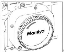
While pressing the lens release button (A) in, rotate the cap counterclockwise, and align the groove (B) on the cap's side with the lens alignment dot (C) on the body. The body cap can then be pulled out.
