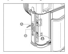
While depressing the back cover lock button A, simultaneously push down the lock lever B in the direction of the arrow and the back will open. When closing the back cover, securely press both comers until it clicks.
