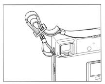
Pass the neck strap through the carrying strap lugs, and fasten it as shown.
