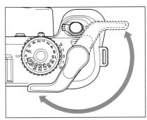
After completing the last exposure, wind the advance lever several times until the film with its backing paper is completely wound onto the take-up spool. The advance lever will become easier to actuate when the film has been completely wound on the spool.
