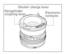
Be careful not to damage the rangefinder coupling lever and the shutter cocking lever at the rear of each lens.
