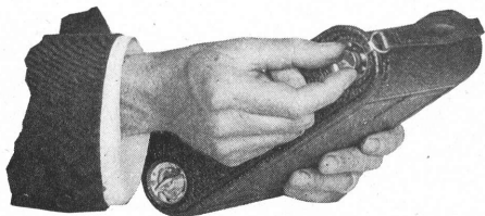
FIG. III. Pulling out Center Pins to remove Empty Spool.
