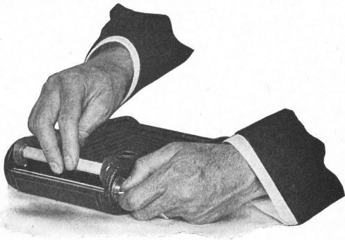
FIG. IV. Pulling out Key to admit new Reel.
