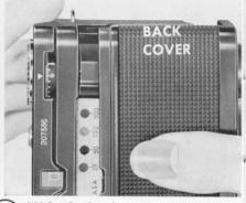
Just rotate the grooved button at the bottom of the camera counter clockwise to align the red dot with "O" (open). This unlocks the back cover.
