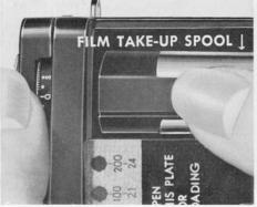
Rotate the film take-up spool with your thumb so that the split metal band is shown as pictured above.
