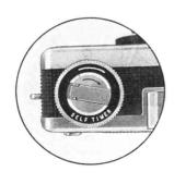
For exposures longer than 1/30 sec., move the Lens Opening Ring off Automatic to the Lens Opening you're going to use. Then, move the Shutter Speed Slide to the "B" position. Swing the Film Advance Lever to advance the film and wind the shutter. Now, the shutter will remain open as long as the Button is depressed, and
