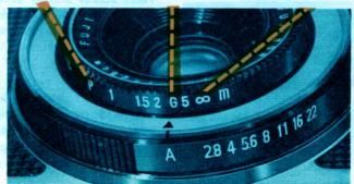
How to switch from automatic operation to manual control and set any combination of shutter speeds and lens openings you wish
