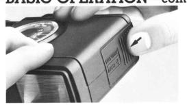
**3.** Close the battery chamber. Slide the lid back into place.
