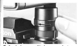
5. Lock the speedlight securely into place.
