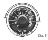
tance is greater, but the recycling time of the speedlight is shorter. On the other hand, the smaller the aperture, the greater the depth of field, but the recycling time is longer and the maximum shooting distance is less. Therefore, in choosing an f/stop, all these factors should be taken into consideration.
