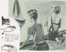
b If no reading is obtained (or reading is very low), open hinged cover at front of hood and read value of light indicated.
