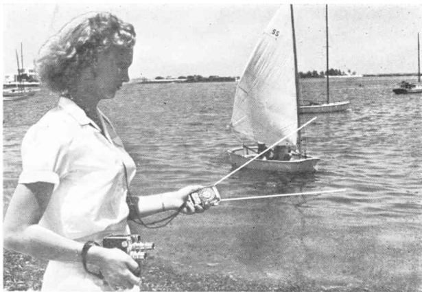
FIG. 6 — For maximum accuracy, hold meter to avoid too much light from sky entering photoelectric cell.
