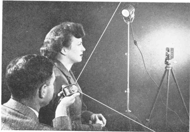
FIG. 3 — For incident light readings, drop baffle, hold meter close to subject, and point at camera.
