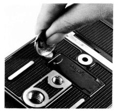
**b** To load the battery, insert a coin into the battery chamber opening button on the bottom of the camera and turn it in the arrow direction
