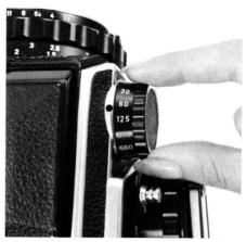
\* If the shutter button is depressed with the shutter speed selector at an intermediate speed, the shutter remains open, and the film shutter knob/crank cannot be turned for the next exposure. As long as this condition exists, battery power is consumed. To make correction, return the selector to the correct setting. Always make sure the shutter speed selector is positioned at a full setting.
