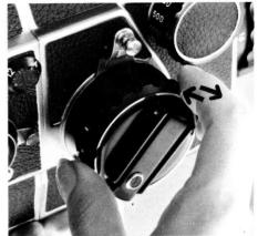
\* The crank stops after it is turned twice, but if additional pressure is applied downward it will continue to turn. This is not a malfunction but the operation of a special safety feature. Applying additional pressure after the crank stops following two full turns is not recommended.
