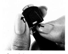
**a** To attach the strap to the camera, press and hold down the spring plate on the strap metal, as shown in the photograph, and slide the plastic holder toward the strap using the metal protrusion atop the plastic holder. The hole on the reverse side of the plastic holder opens. Insert the neck strap stud on the camera body into this hole, and pull the strap toward you, locking the strap onto the neck strap stud.
