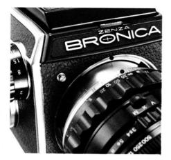
**b** The large bayonet mount accepts such interchangeable lenses as the 105mm lens, 300mm lens, 400mm lens, 600mm lens, 800mm lens, and 1200mm lens. To attach any one of these lenses, insert the lens, align the red dot on the large bayonet mount and the red dot on the lens, and turn the lens fully clockwise until it stops, at which time the focusing ring release but on pops out to its original position. The procedure for replacing the focusing ring is identical to procedure for lens mounting.
