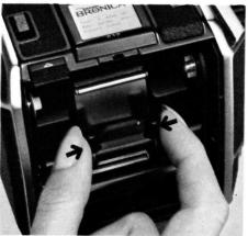
**b** Opening the back cover of the film back reveals the film holder insert, which has two center-positioned knobs. Press these inward, releasing the lock, and remove the insert from the film back body.
