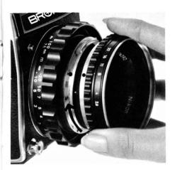
**b** To mount a lens, turn the focusing ring fully clockwise, align the red dot on the lens and the red dot on the mount, and turn the lens clockwise until it click-locks into place.
