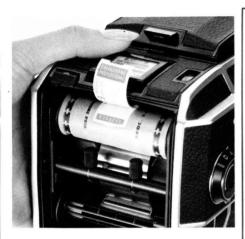
**g** After the 12th exposure with 120 film or the 24th exposure with 220 film, the shutter is freed from the cocking function, and turning the film shutter knob/crank advances the film only and permits winding the leader paper of the film to the end. Open the cover of the film back only after winding up all of the leader paper.
