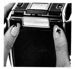
**g** Close the film back cover by pushing the top of the cover against the film back body. It will snap-lock close, completing loading.
