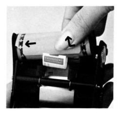
**k** To remove the exposed film, remove the film holder insert from the film back while carefully grasping and holding the loose film. After removing the film seal it.
