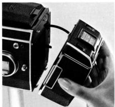
**b** To attach the film back to the camera body, set the bottom of the film back on the open hinge on the camera bottom, after which withdraw the dark slide.
