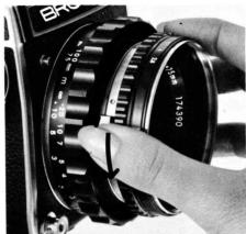
**c** To remove a lens, turn the focusing ring fully clockwise, press and hold the lens release lever with the thumb on the left-hand side of the lens, turn the lens to the left (counterclock-wise) until it stops, and withdraw the lens
