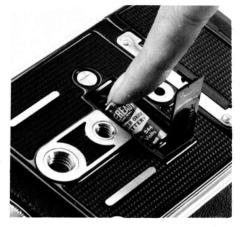
**c** A red "+" mark and a blue "-" are stamped inside the battery chamber. Insert the battery matching these marks with the "+" and "-" marks on the battery, placing the negative side of the battery into the chamber first, pushing the positive side into place, and then closing battery chamber cover. The shutter will not operate if these polarity marks are mismatched.
