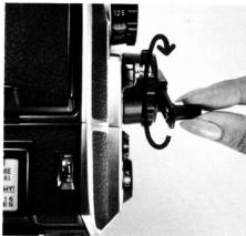
**h** To bring the film to the first frame after loading, turn the film shutter knob/crank until it stops. This advances the film, cocks the shutter, and at the same time advances the exposure counter indication from "0" to "1".
