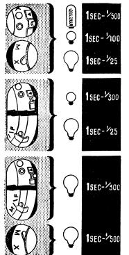
Left: The synchronizing setting determines the shutter speed we can use with flash. The X setting as well as the Vario and Pronto shutters which have only one setting, will synchronize electronic flash at any speed, SM bulbs up to 1/100 sec., and ordinary bulbs up to 1/25 sec.
