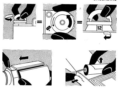
Top: Wind off end of backing paper after last exposure, by turning film winding key until end of paper passes film window, or through five turns where there is no film window.
