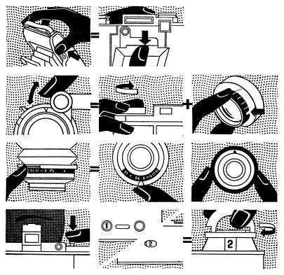
Top: Open camera front by pressing opening button on body (left) or baseboard (right).
