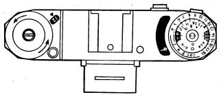
The meter built into the Super Ikonta IV is again similar in principle to the 533/16, but has differently designed scales and the needle window is adjacent to them.
