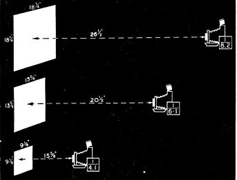
The diagrams indicate the area covered with each supplementary lens, the working distances, and the ratio of reduction (e.g. in the bottom diagram the image on the negative will be approx.  $\frac{1}{4}$  natural size, in the middle one  $\frac{1}{6}$ , etc.). Top, camera and Contameter with  $26\frac{1}{2}$  in. (67.2 cm.) lens; centre,  $20\frac{1}{2}$  in. (52 cm.) lens; bottom,  $13\frac{3}{4}$  in. (34.6 cm.) lens.
