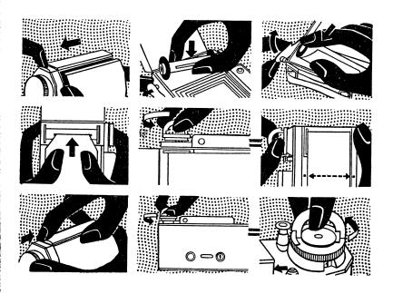
Top row: Open camera back (left), transfer empty spool to take-up end (centre) put full spool into feed chamber (right).
