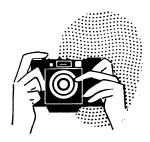
$2\frac{1}{4}\times 2\frac{1}{4}$  in. Super Ikonta (all models). Hold against the nose, the right hand gripping the body, with the right index finger against body release. The left middle finger works the focusing wheel or ring and the left palm supports the camera body.
