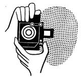
$I\frac{5}{8} \times 2\frac{1}{4}$  in. Super Ikonta. For upright pictures hold the camera with the right hand from above, while the left thumb presses against the body release and the lower part of the camera rests in the arch formed by the thumb and index finger.
