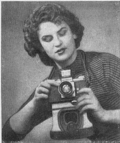
When focusing on the image field lens, hold your Praktica in chest level and take it up close to your eye when using the magnifying lens.
