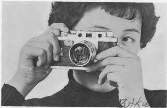
Focusing for the distance with the left hand, releasing the shutter with the right hand
