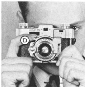
When pressing the lever, hold the breath for the instant. If the Kodak is moved during the exposure, the picture will be blurred. *Hold the Kodak steady.*
