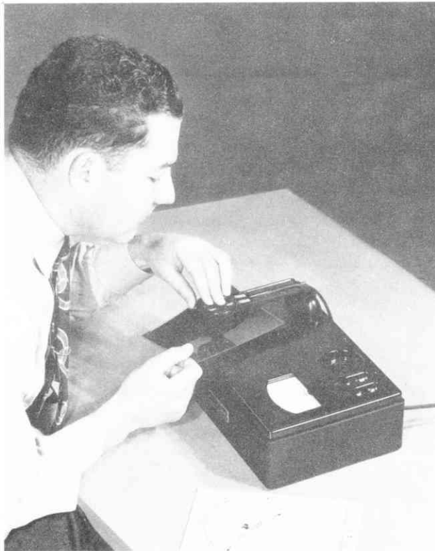
To use as a Densitometer, place negative on viewing plate, and press down the movable arm carrying the Photronic Photoelectric Cell. Fully explained on page 6, and for color separation negatives on page 15.
