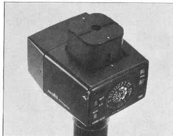
2) Insert Battery Cluster facing triangle marks of Battery Cluster and compartment.
