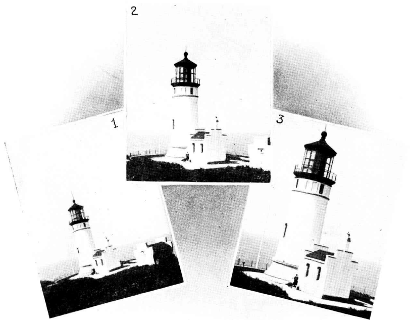
Relative size of image in a picture made with a No. 8 Series VIIa (1) Made with doublet. (2) With rear combination. (3) With front combination.
